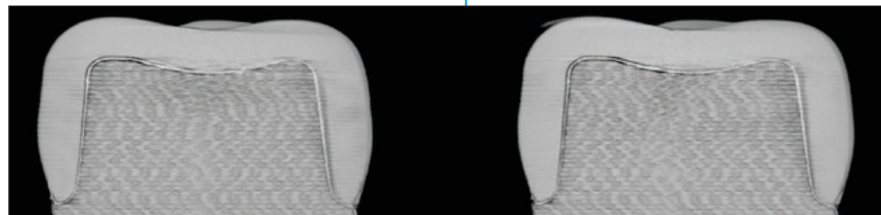
Fig. 11: Comparative \mu CT image (sectional view) of a cemented crown before (left) and after (right) the chewing simulation
