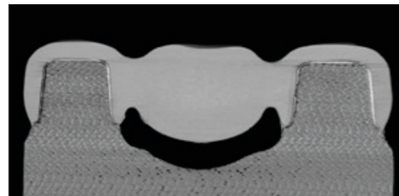
Figure 10: \mu CT image (sectional view) of the cemented bridge after the chewing simulation
