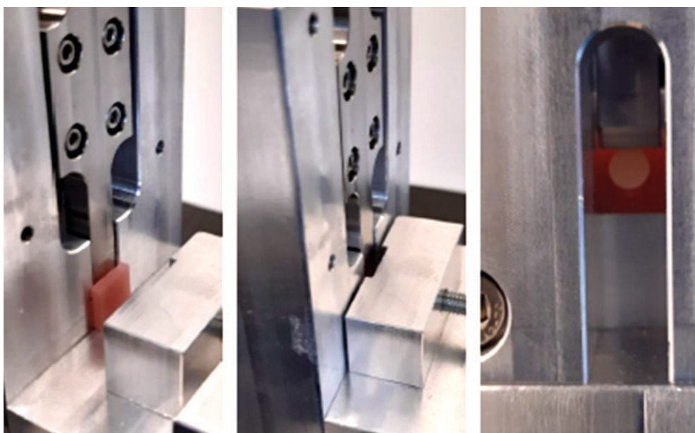
Fig. 18: Test set-up for measuring the bond strength between denture and denture tooth
